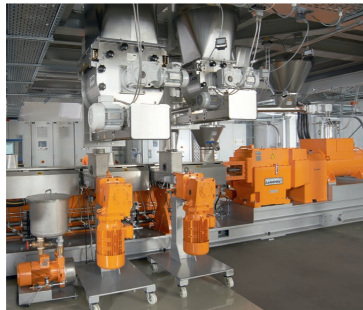
Example of a compounding plant to incorporate calcium carbonate (further details on p. 10/11)
